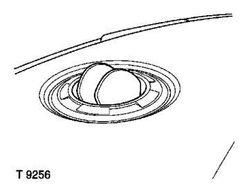
Four ventilation jets are installed in the top of the instrument panel. The ventilation jets may be rotated to adjust the direction of the airflow from the jets.
